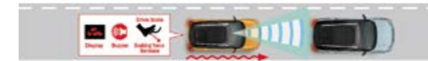
Deploys brake assist to increase braking force if the risk of collision is high and the driver panic brakes
